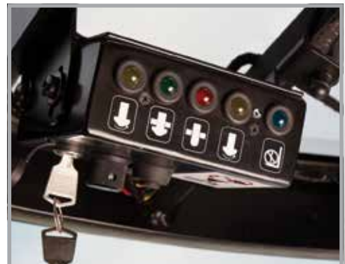
Twistlock module with indicator lights
