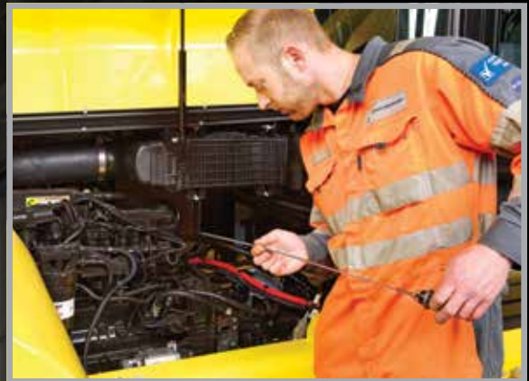
Quick access for engine oil check
