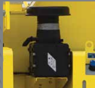
Tier 4 Final integrated pre-cleaner and air filter.
