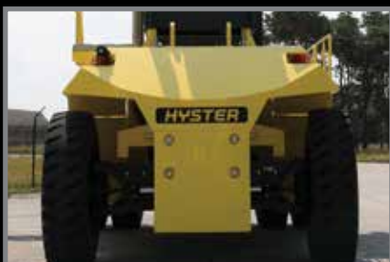
Rear sloping counterweight design.
